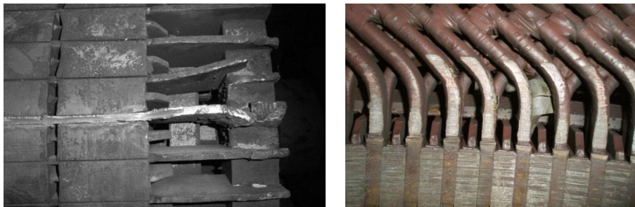
Fig. 2. Damage of the rotor and stator by the broken rotor bars
